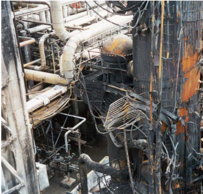
Figure 2. Fully intact Fendolite MII on the left following a directly impacting jet fire.
